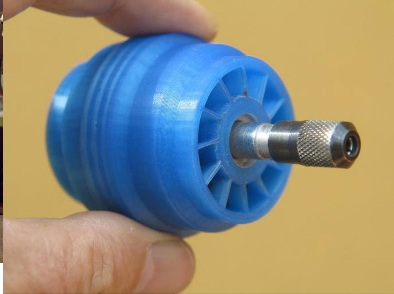
**Fig. 29.** Contributeur RichMac, *Turbine Rotary Tool 60.000 rpm*, 2013, Thingiverse, licence Creative Commons.
